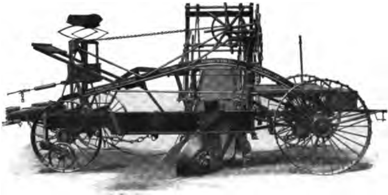
FIG. 11.—Machine for Stripping Topsoil and Grading.
